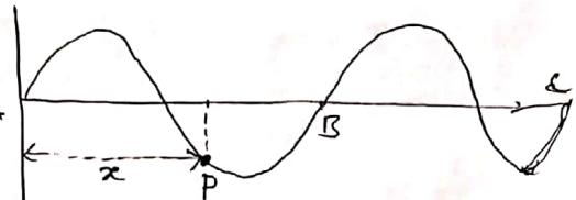
As each particle of the medium executes simple harmonic motion the equation of motion of any particle A, is given by,
