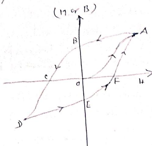
If now  $H$  is decreased, the field  $B$  follows the path AB reaching B at  $H=0$ . The portion OB represents "residual magnetism" in  $M-H$  curve, it is called 'retentivity' and in  $B-H$  curve it is called residual induction. Reversing the direction of  $H$  keeps  $M$  decreasing along BC until it becomes zero at C. The portion OC represents "coercivity" of the magnetic material. Increasing  $H$  in reverse direction produces reverse magnetisation which again reaches saturation at D.
